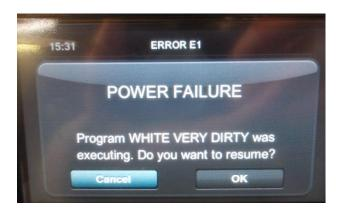
**Caused:** Power shut down during washing.
