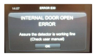
**Cause:** The drum door safety sensor has been tripped.
