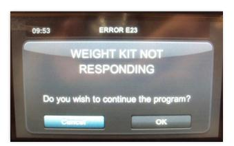
Cause: Values of the weighing block not detected by the CPET card.
