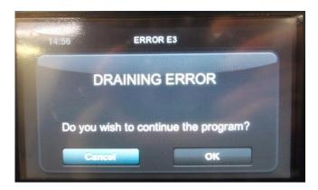
**<u>Caused</u>**: Detection of water in tank during emptying.
