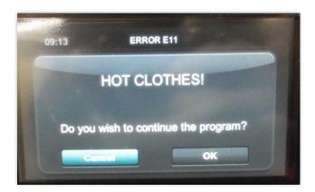
Cause: - The machine was switched off when the temperature was above 50 ° C,
