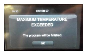
Cause: The internal temperature of the tank reached 95 ° C.
